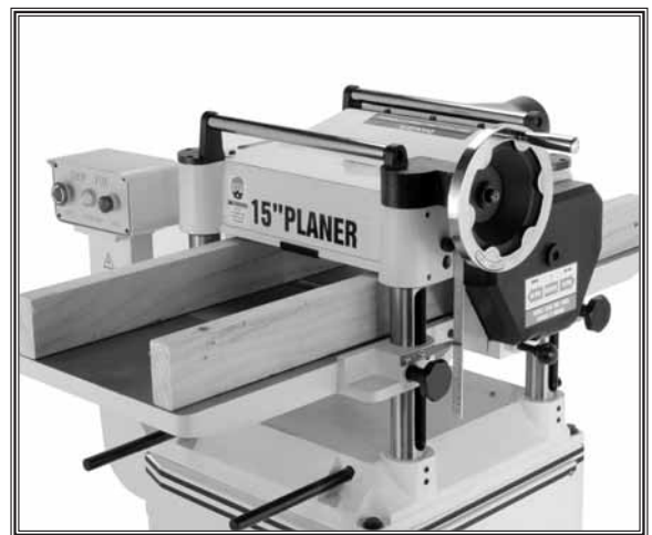
Figure 39. Gauge boards installed.
